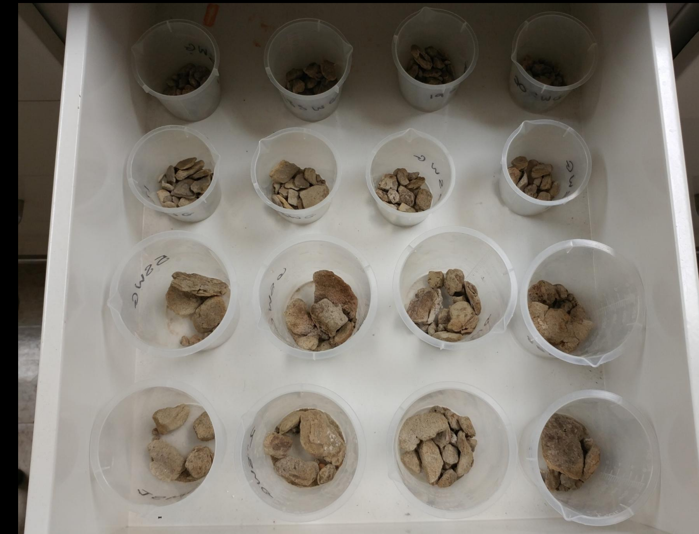
Figure 2: Sediment was weighed and placed into 100mL or 250mL labeled beakers before acetic acid solution was added.
